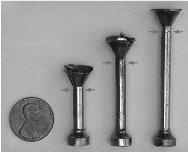
Figure 8.10 Example of cast pins from modified cast pin tear test. The samples are 0.375 in. (9.5 mm) in diameter and have a bottom foot feature. Arrows indicate the location where solidification cracks are normally observed.
